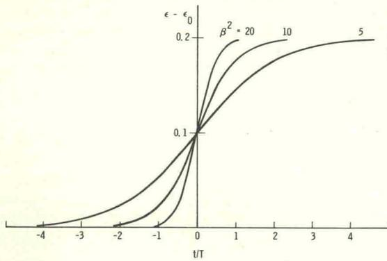
FIG. 4. Steady waveforms of amplitude  $\epsilon_1 - \epsilon_0 = 0.2$  in a material collapsing according to Eq. (20). The effect of increasing curvature in the equilibrium stress-strain curve is illustrated.
