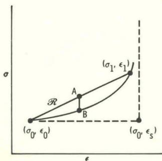
FIG. 2. Typical equilibrium stress-strain curve. Also shown is the Rayleigh line  $\mathcal{R}$  for a wave taking the material from the state  $(\sigma_0, \epsilon_0)$  to the state  $(\sigma_1, \epsilon_1)$ . The dashed lines represent the behavior of an ideal locking material.
