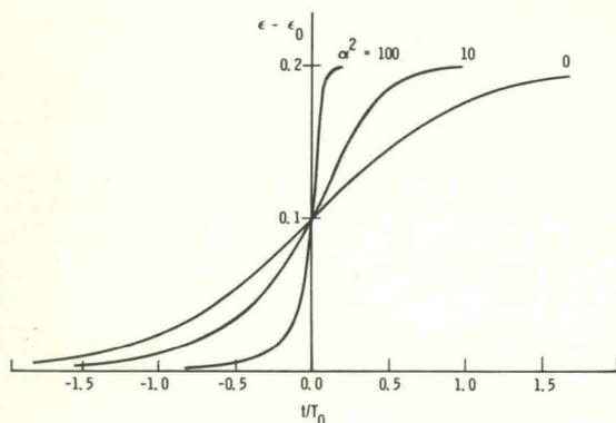
FIG. 7. Steady waveforms of amplitude  $\epsilon_1 - \epsilon_0 = 0.2$  in a material collapsing according to Eq. (24). The effect of increased strain-weighting of the collapse rate is illustrated. We have taken  $\beta^2 = 10$ .
