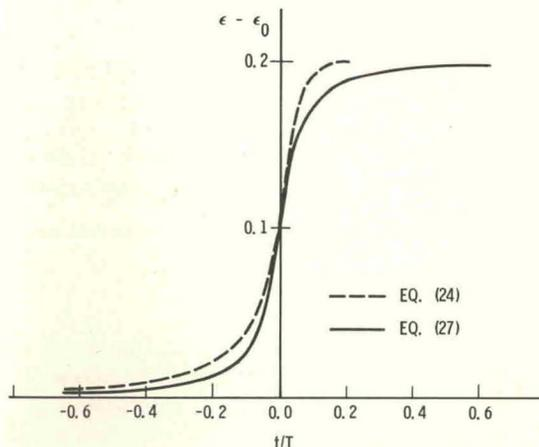
FIG. 8. Waveforms of the same amplitude and rise time calculated according to Eqs. (24) and (27). We have taken  $\beta^2 = 10$ ,  $T_0 = T_1 \equiv T$ ,  $\alpha^2 = 100$ ,  $T_2/T_1 = 0.00887$ , and have  $\tau/T = 0.4459$ .
