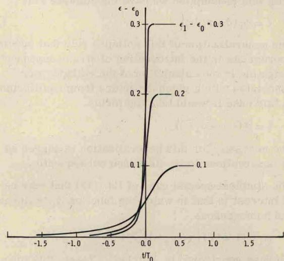
FIG. 6. Steady waveforms of various amplitudes in a material collapsing according to Eq. (24). We have taken  $\beta^2 = 10$  and  $\alpha^2 = 100$ .
