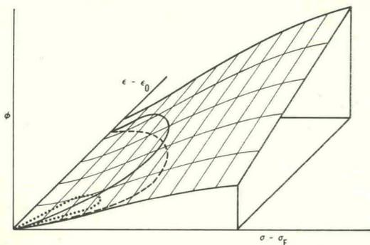
FIG. 10. Typical compaction surface  $\dot{\epsilon} = \phi(\epsilon, \sigma - \sigma_E)$ . The path on the surface shown as a heavy solid line is the locus of  $(\epsilon, \sigma - \sigma_E, \dot{\epsilon})$  states taken at a material point during the passage of a wave. The dashed line is the projection of the path into the  $(\epsilon, \sigma - \sigma_E)$  plane, and the small dotted loop is its projection into the  $(\sigma - \sigma_E, \dot{\epsilon})$  plane.
